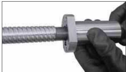
(2) Attached the mandrel towards machine ends.
