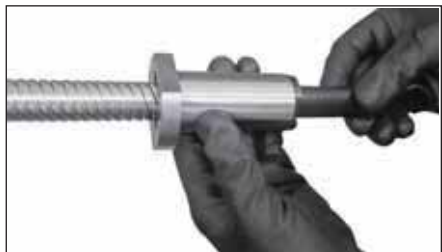
(3) Rotate the ball nut into the screw along the thread.
